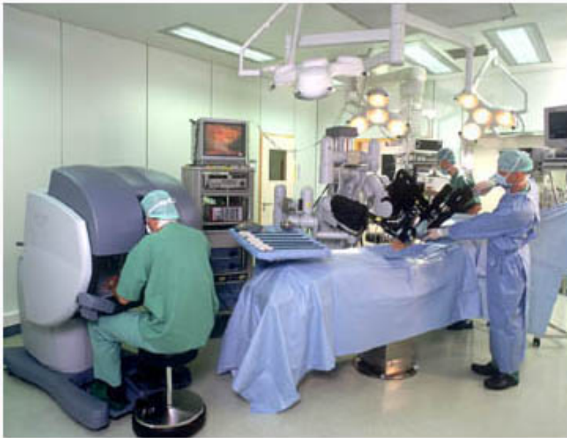
In the da Vinci system, the surgeon sits at a viewfinder (left) and remotely manipulates probes and instruments on actuator arms over the operating table.
